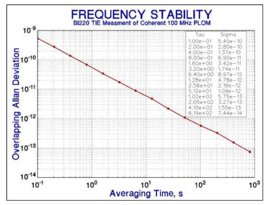
Figure 6. Frequency Stability: 5.5x10<sup>-11</sup> 1-Second White PM Instrument Noise Floor Consistent with that of the Figure 3 frequency measurement.
