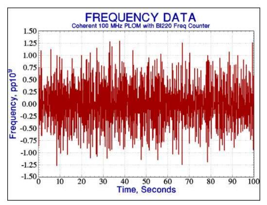
Figure 2. Tau=0.1 Second Frequency Data The average frequency is exactly 100 MHz thus verifying the instrument accuracy.
