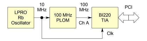
Figure 1. Test Setup – Coherent 100 MHz Phase-Locked Oscillator Multiplier This coherent arrangement measures the noise floor of the measurement system.
