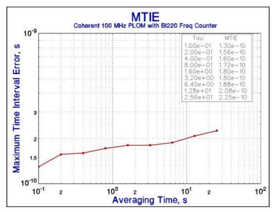
Figure 4. MTIE of Integrated Frequency Data The frequency data has zero dead time so it can be used in this way.
