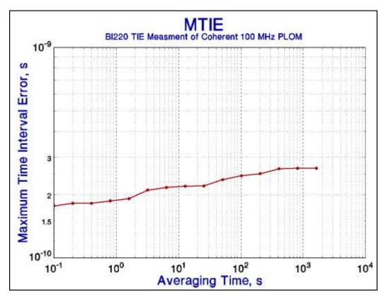
Figure 4. MTIE of TIE Data: 0.19 ns at 1-Second Instrument Noise Floor
