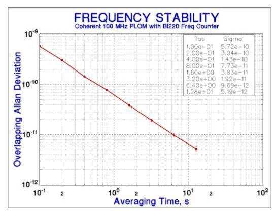
Figure 3. Frequency Stability – White PM Instrument Noise Floor White PM noise is expected from the BI220 analog interpolation circuits.
