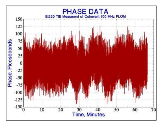
Figure 5. Tau=0.1 Second TIE Data TIE data is preferred for an MTIE measurement
